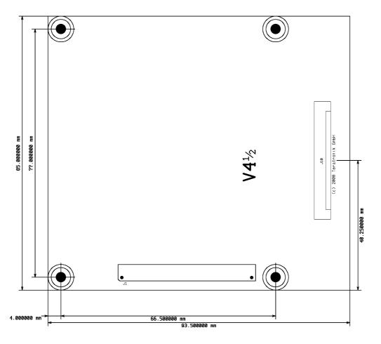
J1 - 120pin board to board connector J10 - 60pin display connector (TTL-RGB)
