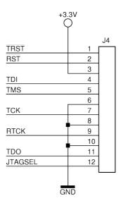
Only mounted on development boards. Adapter to standard 20pin JTAG header is available on request.
