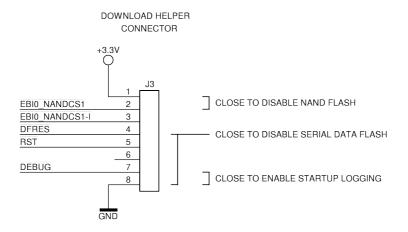
Used to temporary disable on board flash memories. Useful for 'reviving' a dead board that was bricked by loading it with a malfunctioning software.
