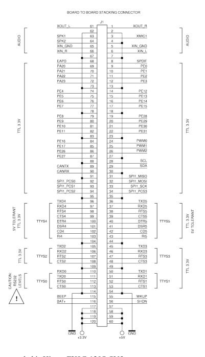
The mating connector needed is Hirose FX8C-120S-SV5.
